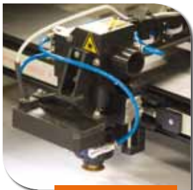
CCD camera kit for registration of cutting to printing markers
