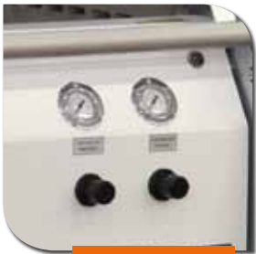
Two level assist gas Kit for cutting/marking
