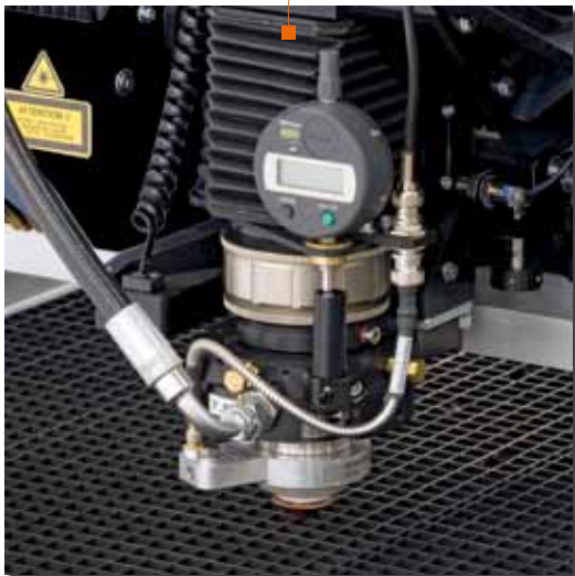
Cutting head with H.P. capacitive sensor
